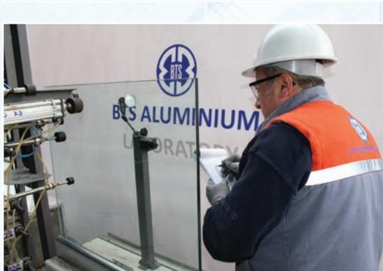
**Horizontal Static Load Test**
